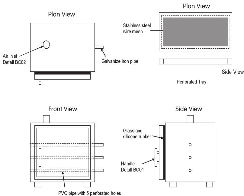
Fig. 1: Schematic diagram of tray bioreactor for SSF
